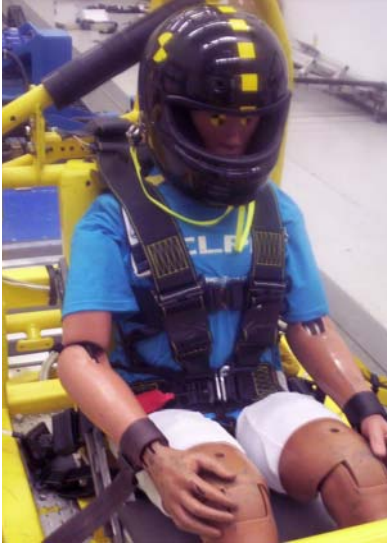
Buckle attachment to Seat Belt System
